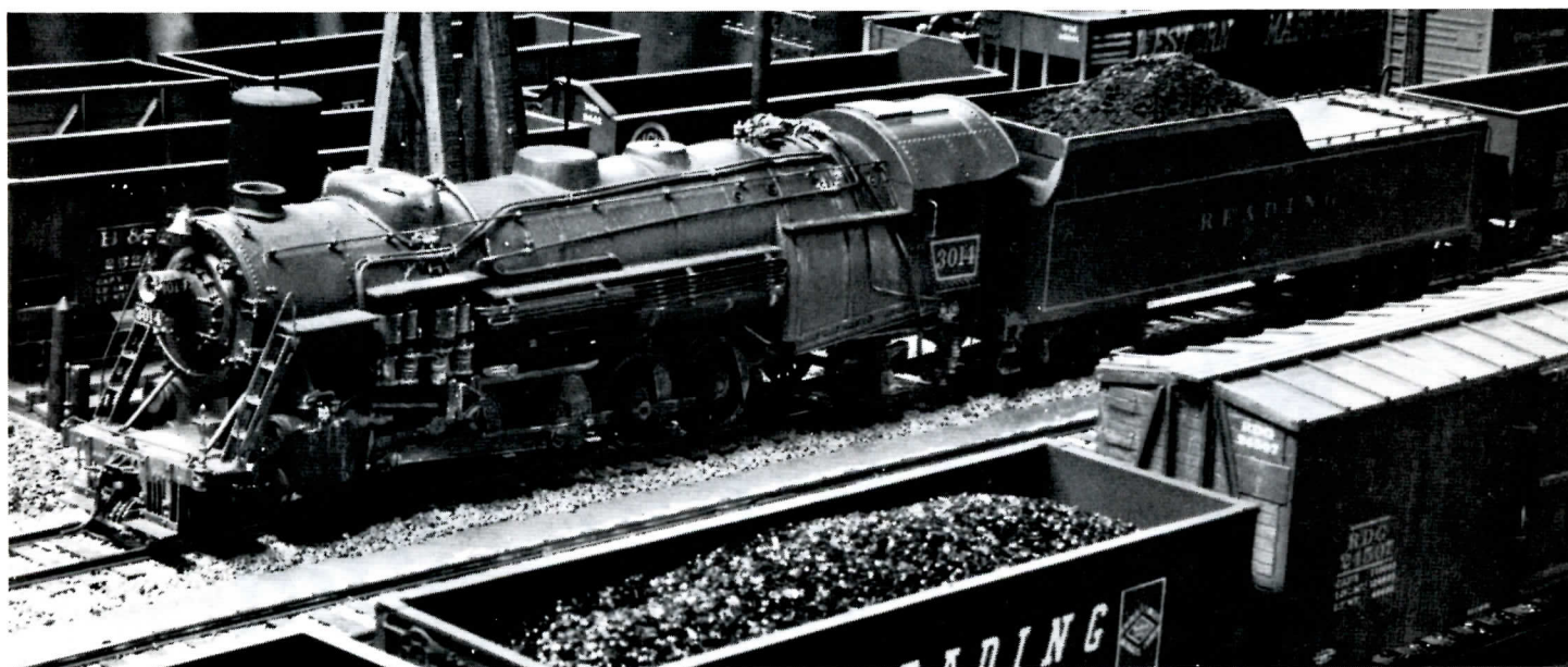
Frank Titman built this rugged-looking Reading 2-10-2. We're guessing that he used a Flyer plastic cab and firebox, Nimco tender trucks, and a mechanism and lots of parts from S Scale Loco & Supply.
