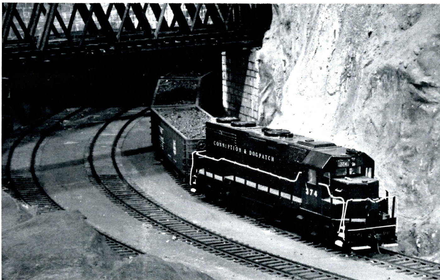
A scratch-built GP-35 with a coal drag passes under Karl Goettert's scratch-built truss bridge. Deceased member Al Dawson did the GP-35 photoengravings in sheet zinc from Model Railroader plans. Hopper cars are AF "triple" bodies with Ace trucks.
