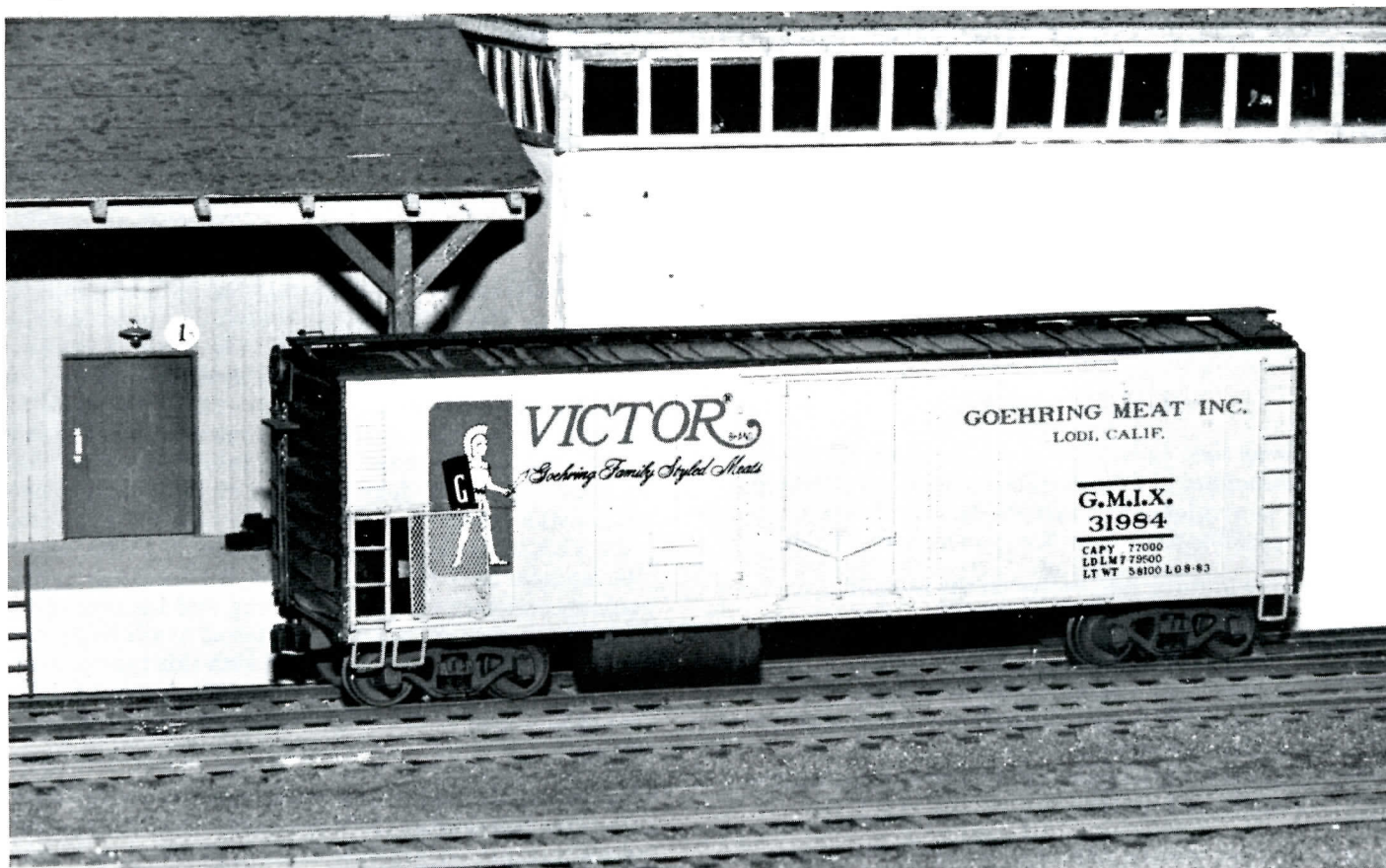
Gale Irwin converted this American Models plug-door boxcar to a mechanical reefer and finished it with Arden Goehring's "Victor" brand dry transfers. Tony Perles (deceased) did the artwork for the transfers. Note the radiator louvers, the open access screen, and the under-floor fuel tank. The building on the left is Gale's low-relief warehouse; the one on the right is Mac McArthur's partially-completed factory-warehouse with walls cast in Hydrocal.
