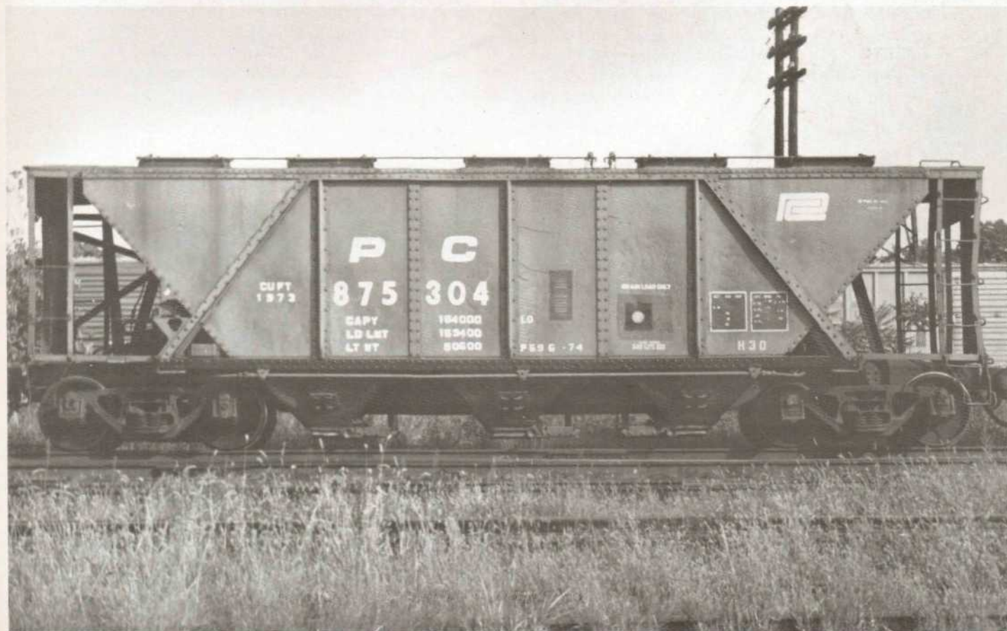
PC 875304 is an old H30 repainted in PC green in 1974. The car's capacity has been increased from the original 70 tons to 77, but this car is stenciled "grain loading only" and it is doubtful that a low-bulk-density item like grain would ever approach this car's weighted capacity. The car is still equipped with friction-bearing trucks, well into the roller-bearing era.
