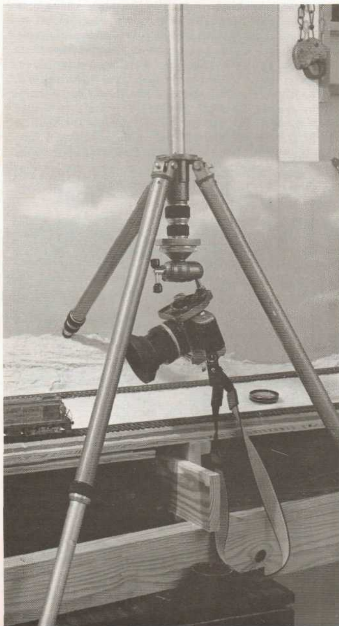
Here we see an innovative use of a tripod to get over the "set." Better tripods like this Gitzo are sturdy, offer individual leg spread, and let you reverse the column for these downunder shots.
