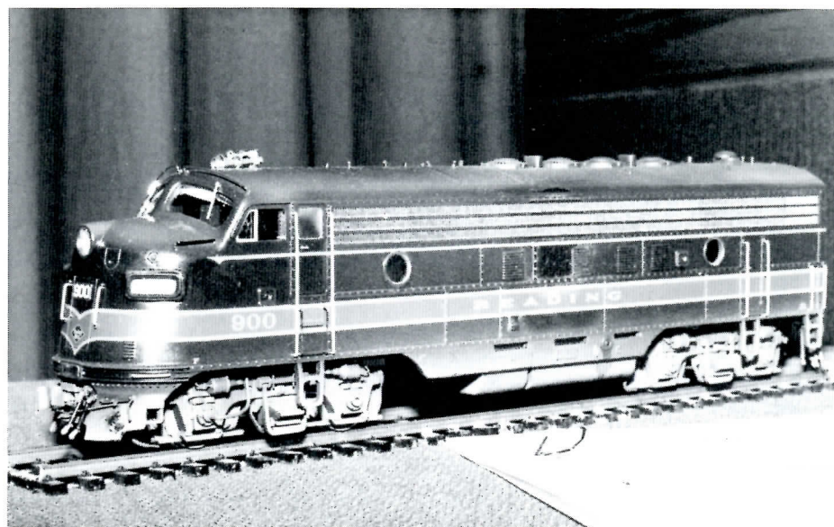
Bill Geracci added to, and altered an American Models FP-7 to turn it into Reading #900. It won first place in the Master Craftsman Diesel & Electric Locomotive category. It has new rear end, flush front door and a reshaped pilot.
