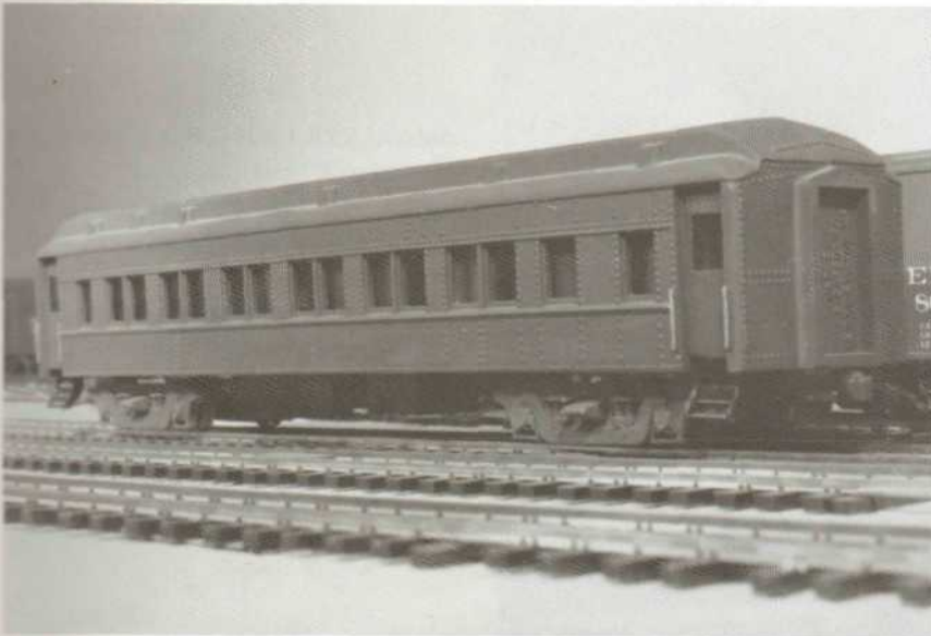
A "Tinscale" Shabbona heavyweight coach with altered window panels ala Nicholson. Bob cut paired window sections from a scrap shell and spliced into this one for a Pullman style arrangement. Two cars are done this way.
