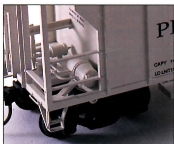
Brake cylinder includes reservoir, ABD valve, brake lever and brake support.
