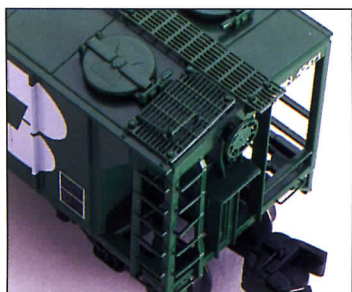
Blau-Knox roofwalks are made of photo-engraved brass, complete with end platform and hand grab.
