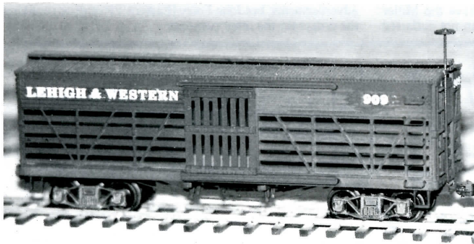
This stock car was converted from an MDC (HO) Old timer stock car. New S brakewheel, etc. Trucks are regauged MDC archbar - 4' wheelbase in S.
