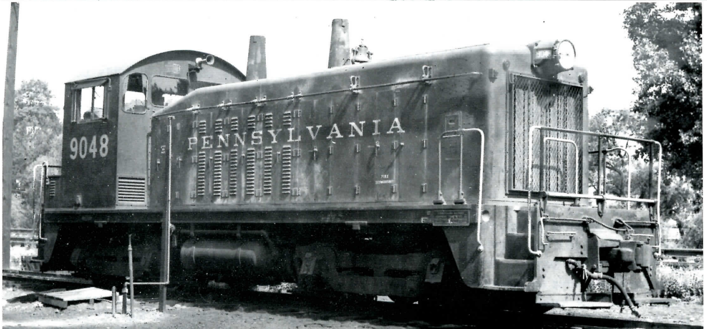
Comparing the upcoming SW9 from S-Helper to the photo above of a PRR SW7, note that the SW9 has no upper vents along the hood. This was the Jeannette, Pa., dedicated local switcher which is shown here in 1972. It replaced a venerable Baldwin which was the former mainstay.
