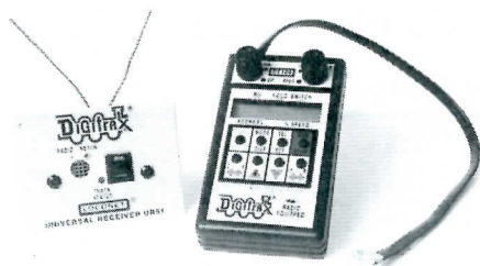
Top left - Digitrax UR91 receiver and DT100R radio controlled throttle. Dangling cord is only for battery failure plug in.
