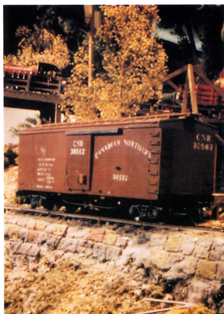
Wooden freight cars with arch-bar trucks and old-time truss rod underframes were typical cars for the time.
