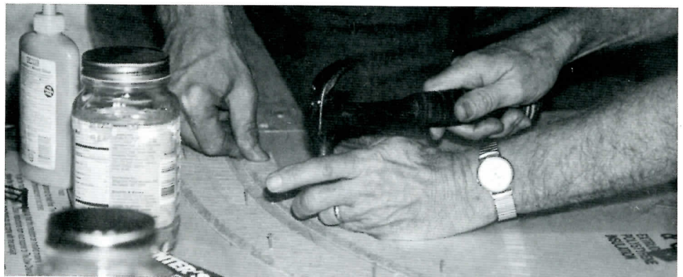
Photo 1: We glued down the Homasote S gauge roadbed as shown. The Homasote non-beveled edge is laid exactly on the track centerline that we marked. The roadbed in this case was laid over a foam sheet, and Elmer's Carpenter's Wood Glue was used to attach the roadbed to the foam.
