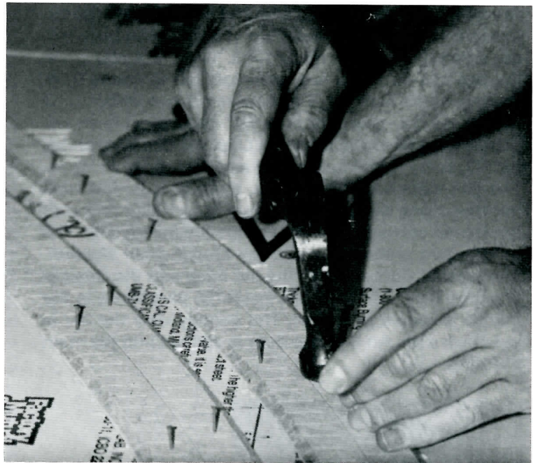
Photo 1: We glued down the Homasote S gauge roadbed as shown. The Homasote non-beveled edge is laid exactly on the track centerline that we marked. The roadbed in this case was laid over a foam sheet, and Elmer's Carpenter's Wood Glue was used to attach the roadbed to the foam.
