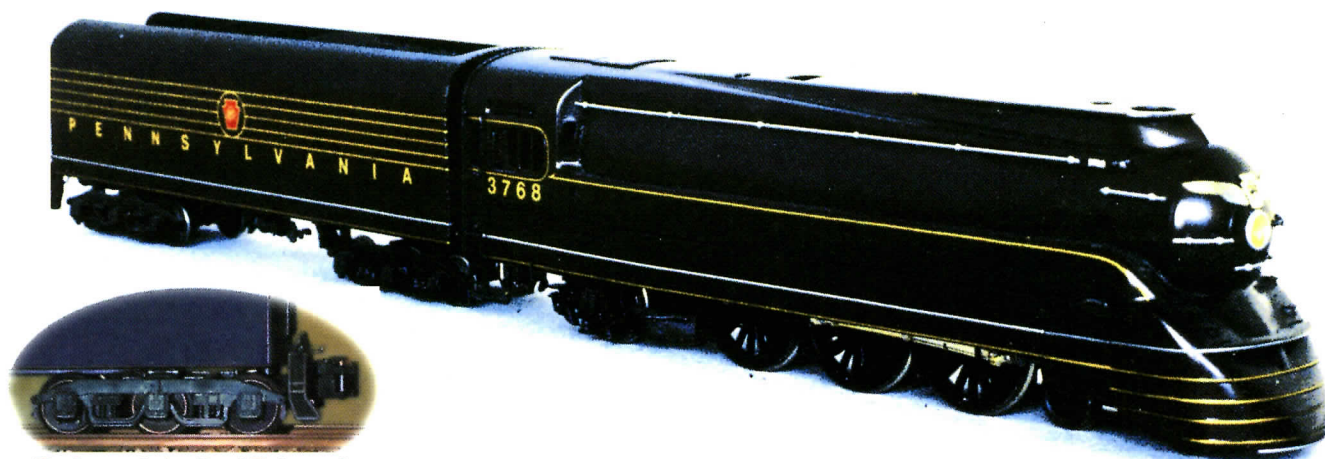
Tender truck details of K-4 sample.
