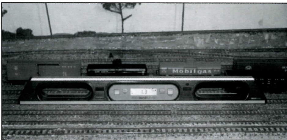
Photo 3. The Smart Level, manufactured by Wedge Innovations, is a very handy tool that digitally reads out grades in degrees, percent, and inches per foot, with a precision of 0.1%.
