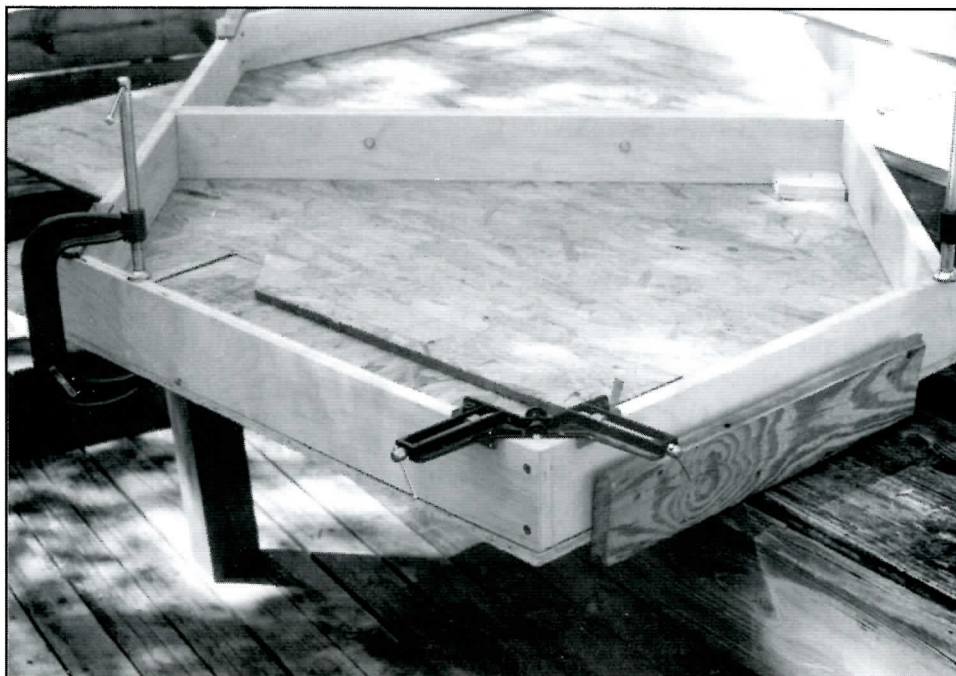
This photo shows clamps used to construct the corner modules. Each 180 degree turn takes 4 modules. Bill Oertly built all 8 needed for the layout to insure uniformity.
