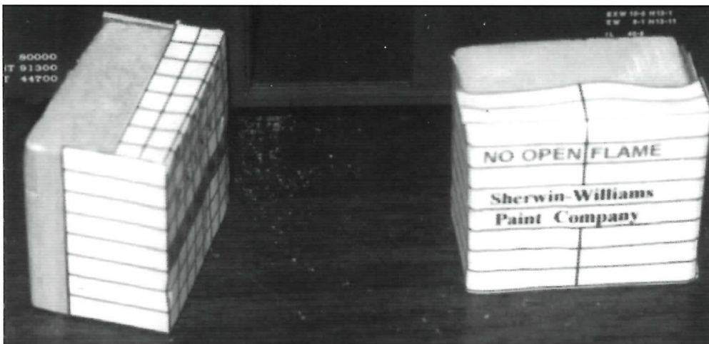
The "Load Sheets" are glued to appropriately sized wood blocks from the scrapbox.
