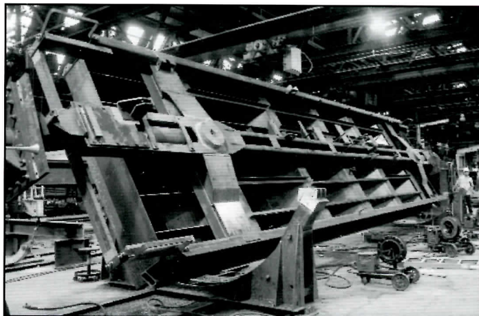
This frame for a "real" 1 to 1 modern coil car is able to rotate 360 degrees for assembly. This was part of the Freight Car America plant tour in Johnstown. Below is a row of finished aluminum hoppers that were assembled at the plant located in the former Bethlehem Steel plant.
