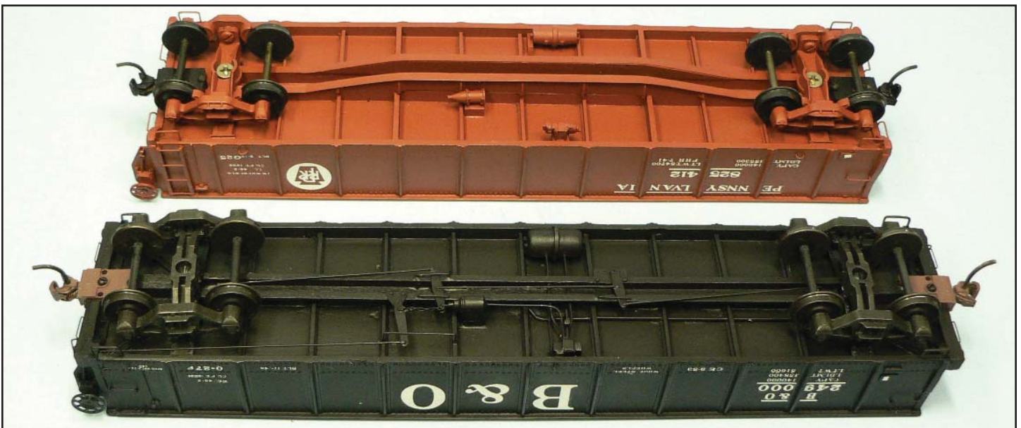
Edwin Kirstatter converted these O-27 Kusan-Auburn gondolas into S scale gons per his article beginning on page 13. Photos by the author
