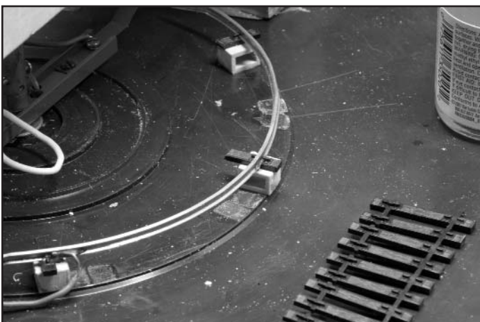
This close-up photo shows how the ring rail is held in place by the cast on spike heads in a piece of Atlas railroad tie. This not only holds the ring rail in place, it also has a little play to accommodate operating irregularities
