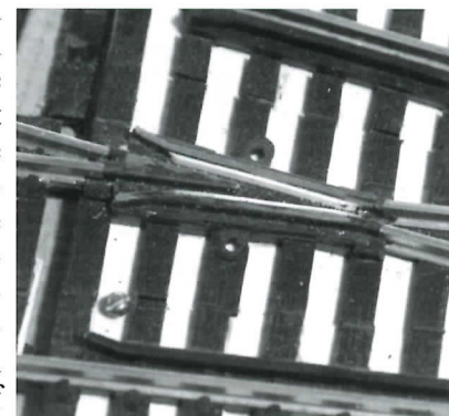
Fig. 5 - .015 x .040” styrene strip will narrow Atlas switch frog flangeways to minimize wheel drop, esp. with code 110 wheels.
