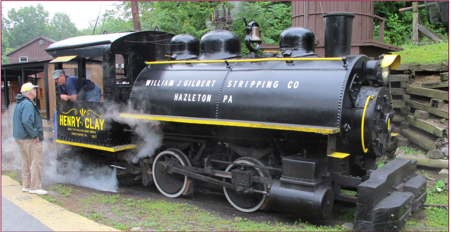
This 0-4-0 Saddle Tank narrow gauge steam locomotive, built by the Vulcan Works in 1927, hauled visitors on a tour of the Pioneer Coal Mine. Photo by Peter Vanvliet
