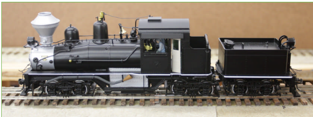
The opposite side of my Sn3 model shows a gray hose on the side for sucking water out of streams, etc. The tan part is a filter to keep fish and large debris out of the water tank. This one is a wood or coal burner instead of an oil burner like the other two models.
