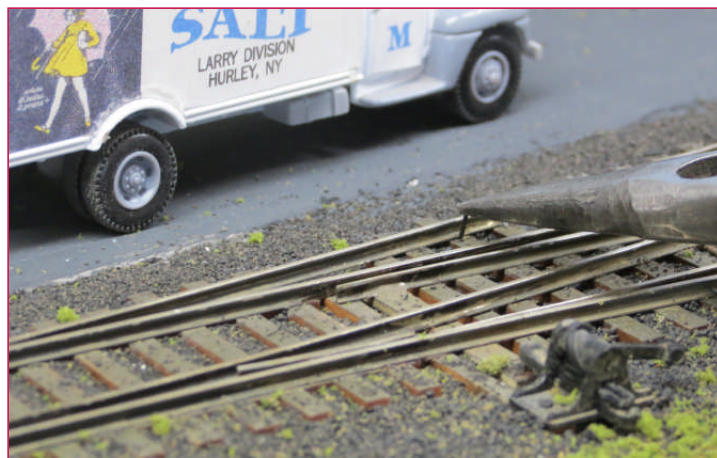
Above and below: Adjusting a tight spot on a three-way turnout by heating the rail and pushing it into the proper gauge. Removing the heat while holding the rail in its new position for 5 seconds, then adding a spike will permanently correct the problem.
