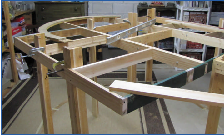
Above: Open grid benchwork for the new peninsula is up on L-shaped legs. The lower staging loops go on this.
