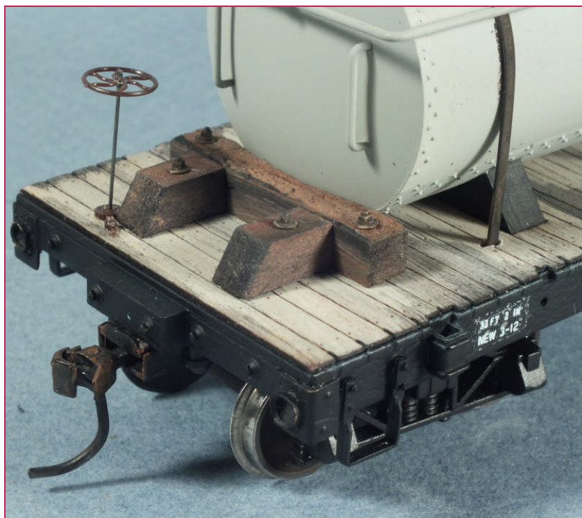
FIGURE 7, below: End bracing was hand made from basswood and NBW castings. The bracing on each of the three cars was varied slightly to provide visual distinction.
