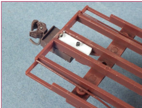
FIGURE 7, below: End bracing was hand made from basswood and NBW castings. The bracing on each of the three cars was varied slightly to provide visual distinction.
