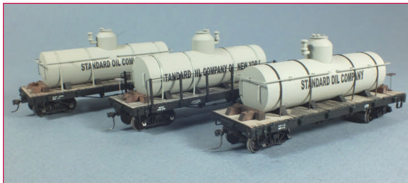
FIGURE 6, above: Three versions of an interesting tank-on-flatcar were built using a Bachmann On30 tank car and a detailing kit from RS Laserkits. The detailing kit includes peel-and-stick decking, a new brake wheel and decals. The side railing on the center car in the photo was made from 1/16" (.0625") square styrene which fit perfectly in the side pockets of the Bachmann car, then drilled to accommodate 1/64" (.015625") brass wire railings.
