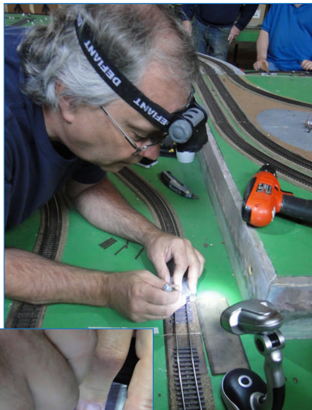
Right and below right: Using a track gauge and a pin vise, Shane Jibben drills tiny holes for tiny spikes.
