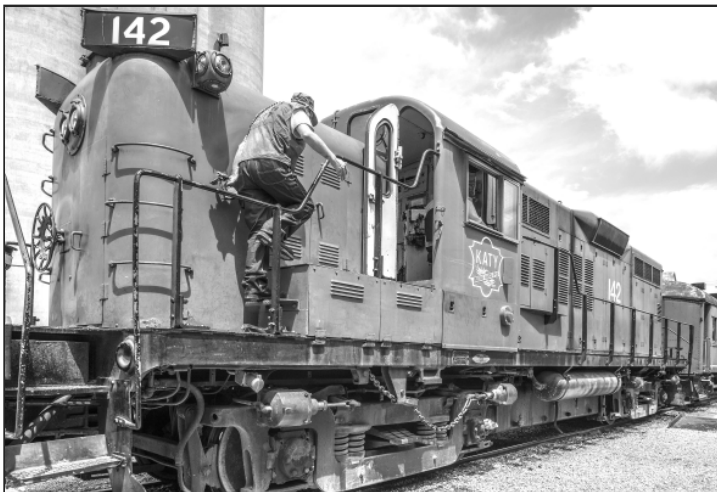
A unique Alco RS-3 loco, rebuilt with an EMD prime mover, hauled our train across the Kansas prairie. Roy Inman photo
