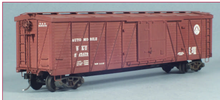
Figure 8: This photo shows the car after painting with Floquil Box Car Red and applying decals from the authors scrap box. The trucks are from Ace and the couplers are Kadee 802s with the glad hands painted black with silver to represent the coupling.
