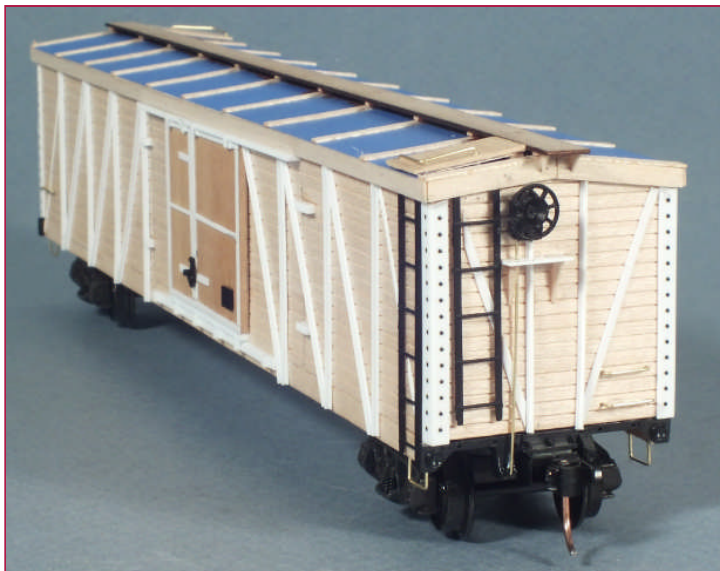
Figure 7: This view clearly shows the angle iron corner braces with rivets represented using Archer Fine Transfers. The ladders and brake wheel are from a PRS kit. Grab irons were formed from .020" brass wire. Blue painters masking tape was used to represent the roofing material and the roof walk is a laser etched part from BTS.
