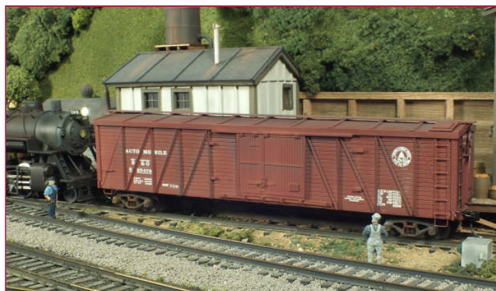
Figure 9: A B&O Consolidation switches the interesting 50' outside braced boxcar the author built from parts from two 40' box car kits manufactured by Huff-N-Puff. New scribed siding, a roof walk from BTS and plastic details completed the transformation.
