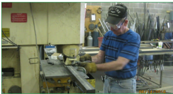
Joe Glenn cutting metal tabs secure leg corner brackets.
