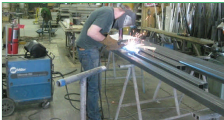
Larry Rascop, master welder, welding leg corner brackets.
