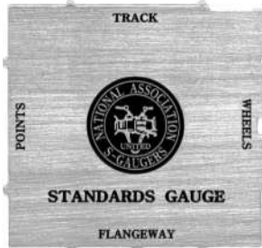
NASG S-3, S-4 TRACK AND WHEEL GAUGE
