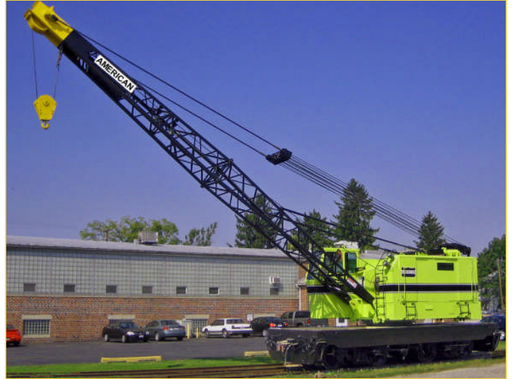
Above: This modern diesel powered crane, manufactured by American Ohio Locomotive Crane Company, is configured to ride the rails. The same crane can be mounted on a truck body and moved on the highways.
