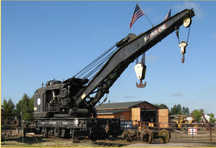
Fully functioning Southern Pacific Railroad Bucyrus-Erie steam-driven crane on display on the grounds of the Antique Overland Transportation Museum at Brooks, Oregon, just north of Salem. Photo by Bill Pyper
