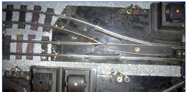
Above and below illustrate the difference between a normal 5-1/8" offset and a modified AF switch with a 2-1/2" offset. Note the modifications to gain the tighter yard ladder spacing. Above switch #19 illustrates the standard AF offset of 5-1/8 inches. Below switch #20 has been modified to an offset of 2-1/2 inches. This modification is described on the next page.
