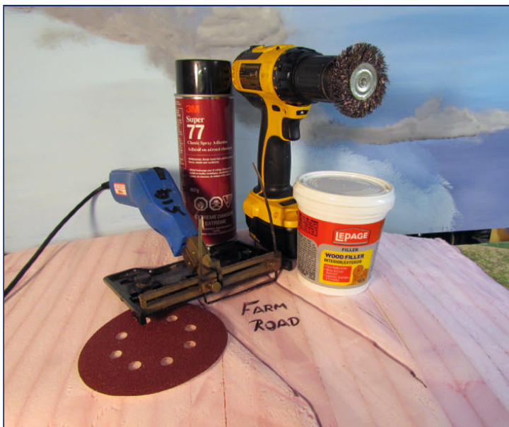
The author's scenery forming tool kit: 60 or 80 grit sanding disc, professional foam cutter, Super 77 spray glue, cordless drill with wire wheel brush, water soluble wood filler.
