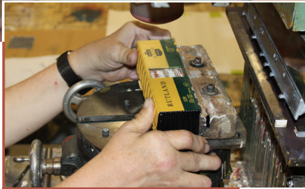
Above and right: Corbin operating the pad printer to decorate a boxcar.
