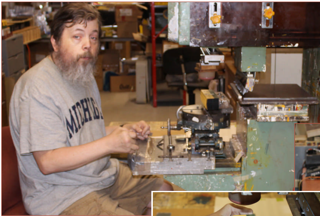
Above and right: Corbin operating the pad printer to decorate a boxcar.
