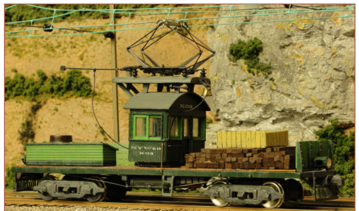
Figure 4, above: If you can't find a Stanton with a suitable wheelbase, surf the NWSL online catalog of other-scale Stantons. Here's an HO 9-foot wheelbase Stanton with S scale 36" wheels beneath my S scale line car. It fits the 7-foot wheelbase of its old Dayton traction sideframes nearly perfectly. For this installation I used CA (cyanoacrolate or Super Glue) to attach a styrene shim to the center of the backside of each sideframe. Then I used Plastruct Plastic Weld to attach the styrene spacers to each Stanton sideframe mount. After the Plastic Weld begins to melt the shim and the Stanton's housing together, you can adjust the sideframe's position for perfect alignment. The four wires connect to a DCC decoder stuffed into the unit's cab (left).
