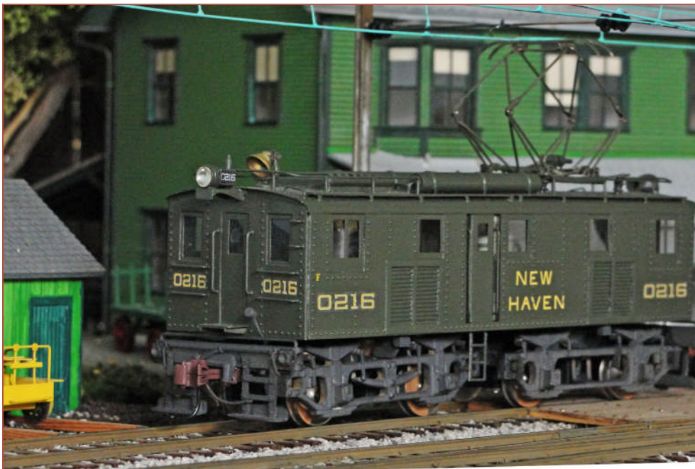
Above: This New Haven Class EY-3 electric yard switcher was custom-built in the early 1940s with a small Pittman open frame motor and a chain drive on just one truck. The author repowered it with two under-the-floor Stanton drives. This locomotive was used for the motor testing described in the text.
