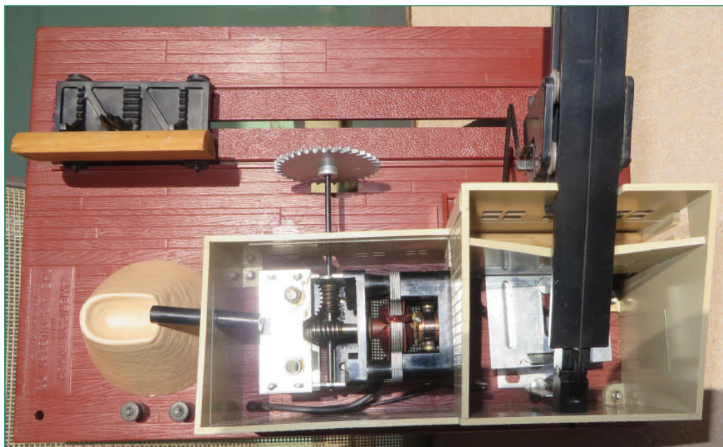
A worm and gear reduces the motor speed for the saw. A second worm and gear reduces the speed of a vertical shaft that goes below the deck. At right is a sliding plate that pushes out one "cut" board each time. The entire mechanism was well designed.
