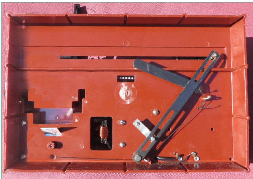
A worm and gear reduces the motor speed for the saw. A second worm and gear reduces the speed of a vertical shaft that goes below the deck. At right is a sliding plate that pushes out one "cut" board each time. The entire mechanism was well designed.
