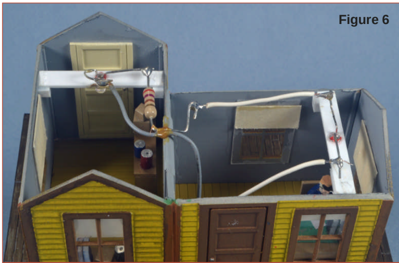
Figure 6: Two LEDs in series with legs bent in opposite directions.
