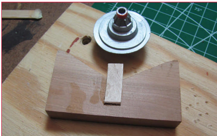
Centering jig with finished turbine and hole in plywood.
