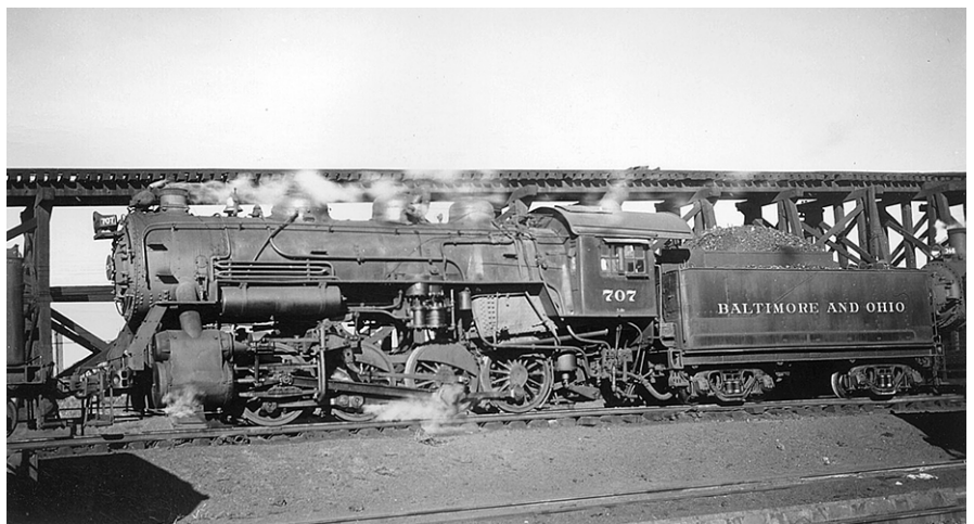
FIG. 2 - This undated photo of B&O Class L-2c #707 was made by Ralph Dunn. The configuration of this engine was typical of the L-2c class and the locations of appliances closely matches the SHS Consolidation. Even the firebox appears light gray!
