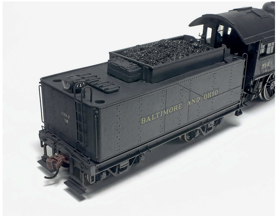
FIG. 7 – Brooks modified the molded coal load from the Consolidation tender to fit in the new coal bunker. A tool box was added to the tender deck.
