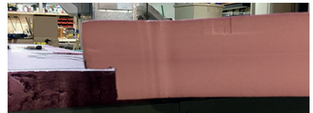
Figure 4: Notching of the foam board perimeter
