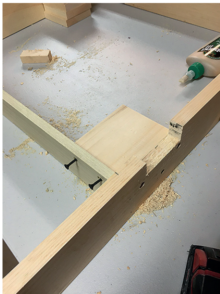
Figure 2A: Leaf Lock notch and support: notch and support block installation, Figure 2B below: installed leaf lock.
