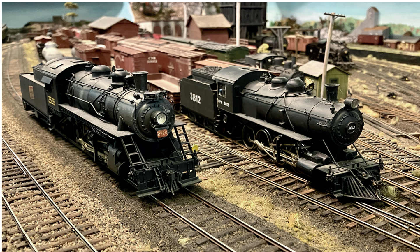
This side-by-side comparison is an excellent example of how Paul backdates his steam loco fleet to 1920. Compare this mostly stock Omnicon 2-8-0 (2526) with the one that Paul has altered (3812) with inboard piston valves, wood pilot, high headlight and simplified boiler piping.
