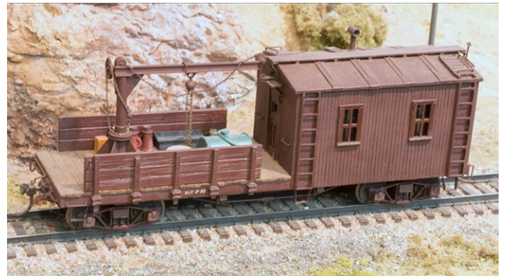
This boom car is one of six MOW car kits offered by Bob Peare Engineering. The builder of this car has added an on-board gantry that disabled its ability to actually be a crane boom tender. Bob Werre photo.
