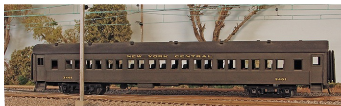
Exacta’s kits of Etched copper sides and ends applied to wood core bodies were among the first metal-clad S scale offerings. This particular car’s roof has been replaced with a detailed arch roof. Trucks are American Models.
