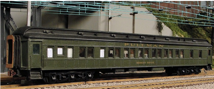
Super Scale passenger-car kits were similar to Exacta's. The 12-section Pullman shown here was built per the kit instructions. The only non-Super Scale additions are the couplers, diaphragms, and AM trucks.
