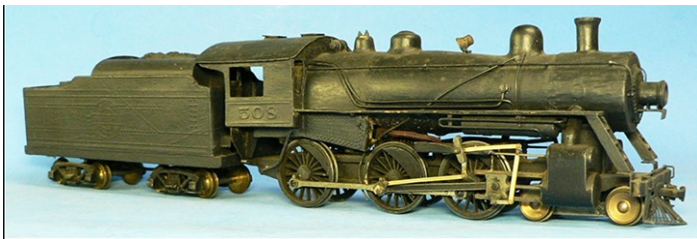
The CD steam loco kits consisted of wood basic body parts, cardstock overlays for cab and tender, a few metal details, powered chassis components, and trucks. The CD Chicago Great Western ten-wheeler shown here was built and photograph by Edwin Kirstatter.
