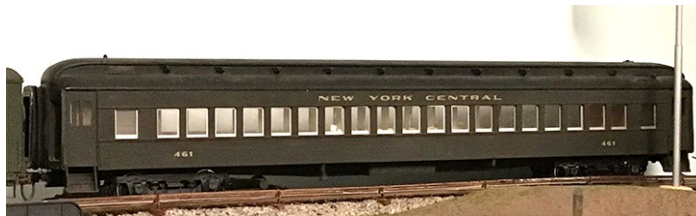
The Nimco coach kit was basically wood with aluminum sides (no rivets), brass doors, celluloid window strips, aluminum sash insert, and soft metal steps and trucks. The Ward vents on the pictured car were fashioned by the modeler.
