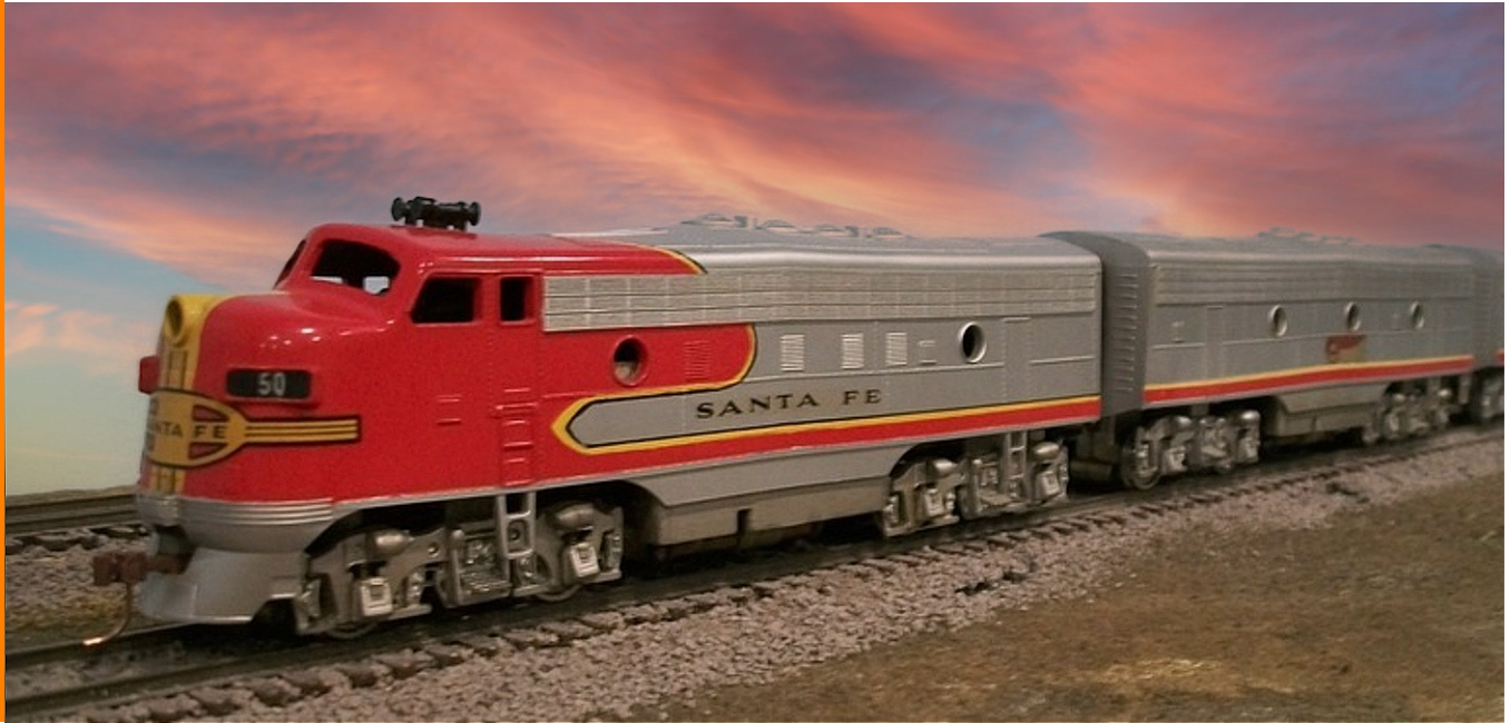
The Enhorning Industries EMD F units' powered chassis design was state-of-the art, but their plastic carbody moldings were unstable over time, developing the obvious roof humps evident in the photo. Jim Syphax photo.
