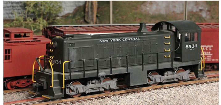
Everything seen in this photo except the trucks was in the original Miller Alco S-4 kit. This model's Miller power trucks have been replaced with NWSL Stanton drives with Smoky Mountain Blunt sideframes, which make it an S-2..
