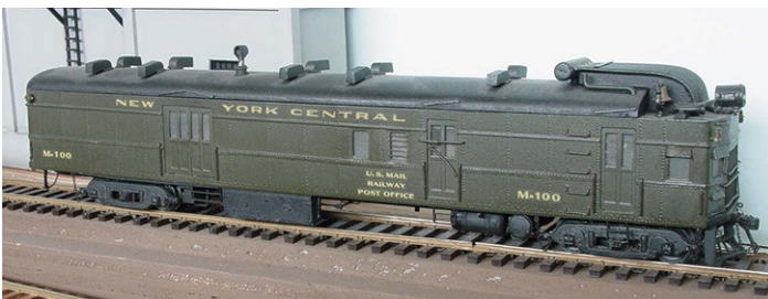
Perhaps Dayton Model Products' finest kit was this New York Central gas-electric. The kit included stamped brass sides and ends, wood roof and floor, wood and white metal details, and a complete power unit. This particular model was built, detailed, painted and lettered by Kent Singer, who replaced the Dayton drive with a Hobbytown HO drive.
