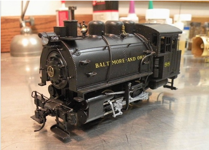
The first Rex Engineering locomotive kit was this B&O "Dockside" 0-4-0T tank engine. The $36 all-metal kit was exceptionally well detailed for 1950s kits. Modeler and photographer Rusty Rustermier added a few extra details, the most obvious being the front-facing windows in the cab, as there were none on the kit casting.
