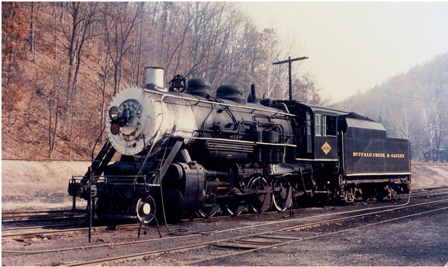
This classic portrait of #4 at the Dundon yard was taken by Howard Ameling sometime after 1959 when the diamond logo on the cab was reintroduced. The basic elements Brooks incorporated in his model are evident including the bell location, red number plate, the pilot mounted air tank, the light smokebox and the white striping.
