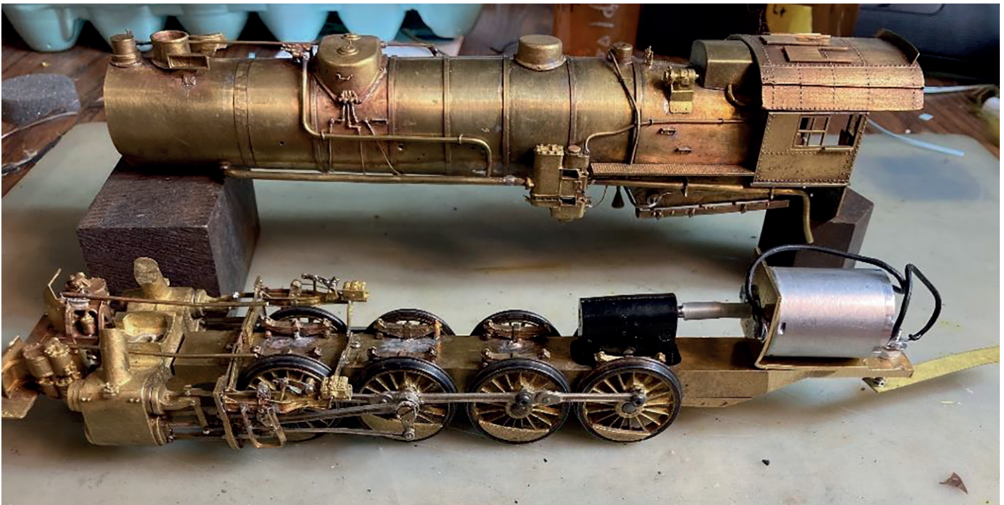
After this photo was taken, Mike determined that a larger motor was required. In order to fit it inside the firebox, he had to move the gearbox to the number three axle which necessitated remilling the chassis, work Mike was willing to do to get a locomotive that would serve its intended purpose for years.
