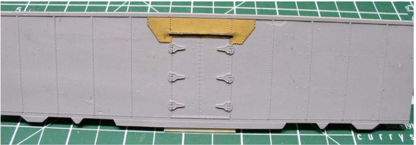
Figure B1b - Later Style of Patch Over Door
