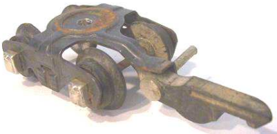
Diecast or plastic link coupler, metal sideframes & plastic wheels (1946-54)
