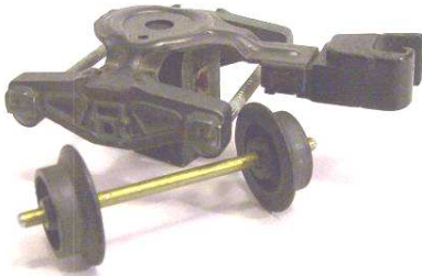
Metal or plastic knuckle coupler on plastic frames & wheels (1952-66)
