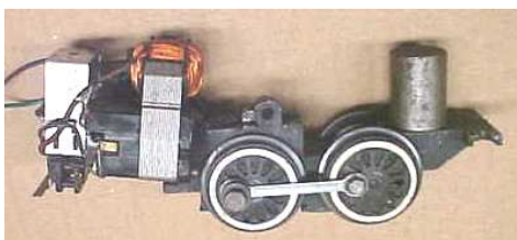
4-wheel frame-worm motor-2pos. rev.
